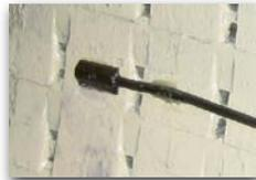
The Iris Power TFProbe has been primarily designed for hydrogenerators and other salient pole machines. This probe can also be used in round rotor machines with air gap size less than 50 mm. The probe sensing element is a small printed board (12 mm wide, 25 mm long, 4 mm thick) which is affixed to a stator tooth with epoxy. In many machine designs, it is even possible to install the probe without removing the rotor – a definite advantage in retrofit applications.
